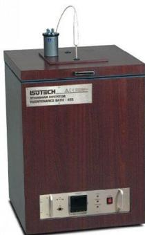
The test resistors are placed in the Isotech Model 455 Resistor Maintenance Bath and allowed time to stabilise. Measurements are then made using the world-leading microK Thermometry Bridge, comparing the test resistor against our own calibrated reference resistors. The microK is used in the world's leading NMIs and has a ratio accuracy of  $< 20$  ppb (unity ratio).
