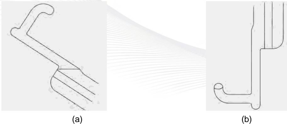
Figure 2b: Procedure for entrapping a gas bubble in Type A cells: (a) position the cell as shown (b) gently invert the cell to trap and compress the bubble.
