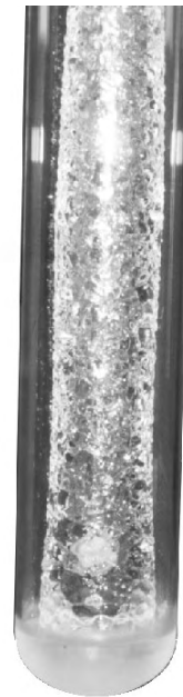
2 K.T.002 The Ice Mantle The Concentrated colour around the Ice Mantle is due to the Ice rejecting the impurities in the water.
