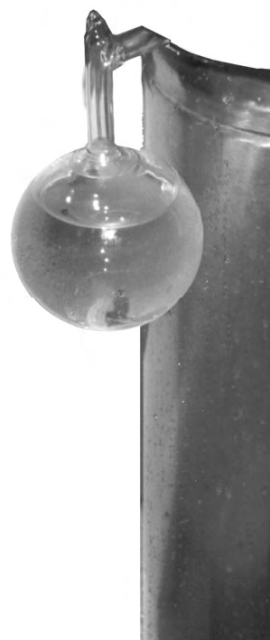
6 K.T.001 The Liquid is quietly distilled back into the cell By placing the cell in crushed ice and leaving the flask at room temperature.
