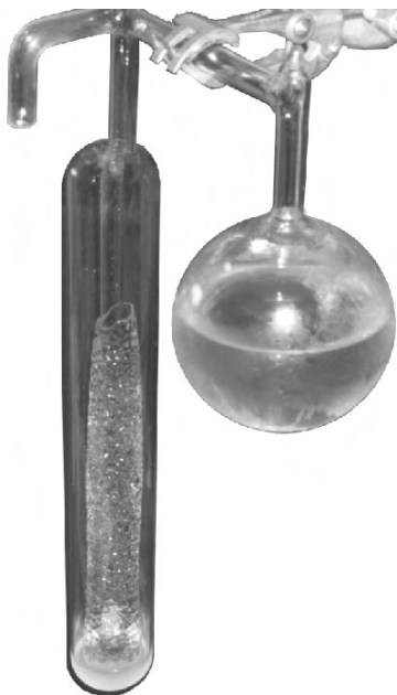
3 K.T.001 After testing the cell The water can be transferred to the flask, leaving behind the pure ice mantle.
